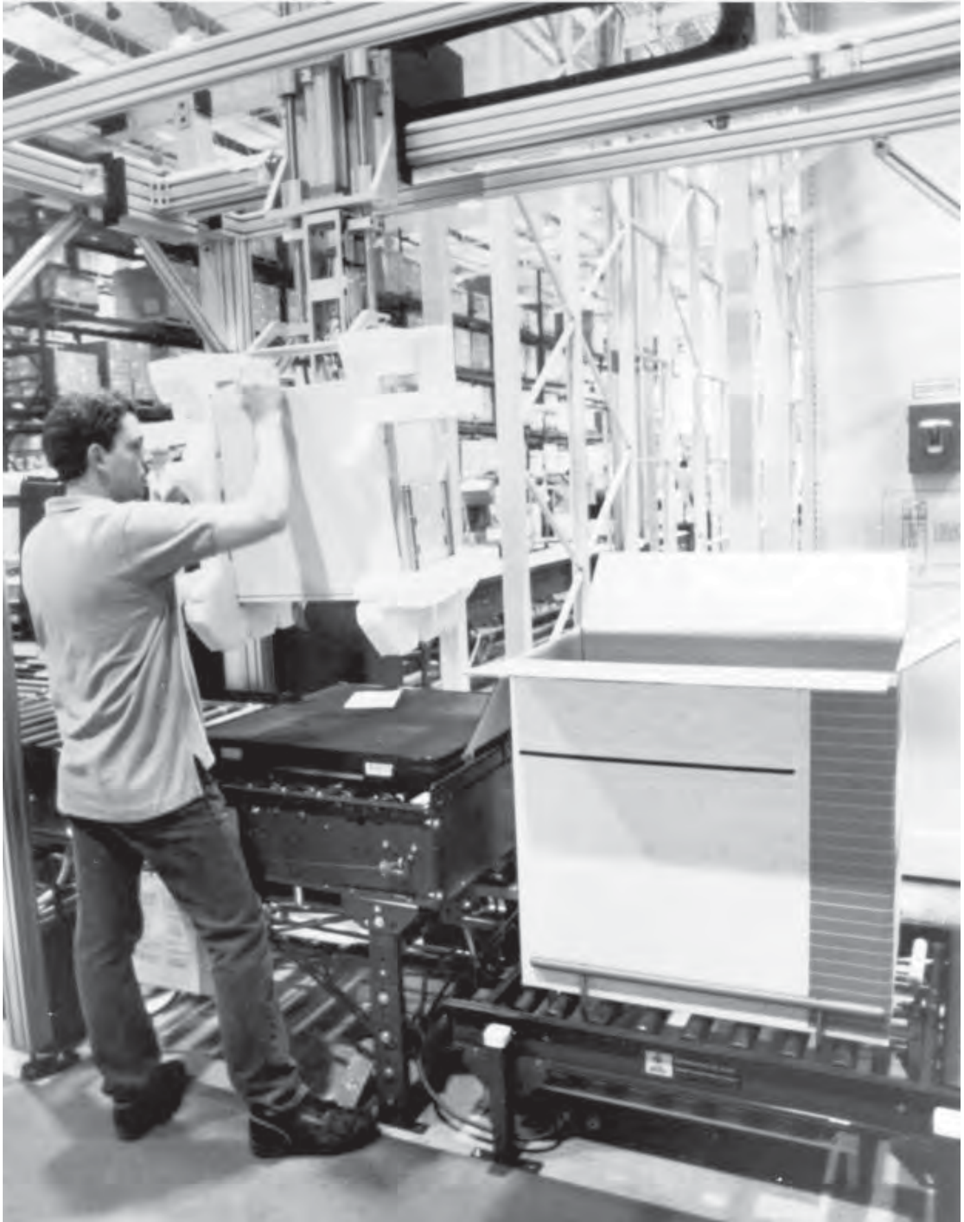
3-Axis gantry loader with vacuum pickup
